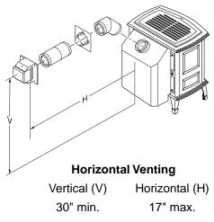
Figure 26 - Horizontal Termination Configuration for Rigid Venting
